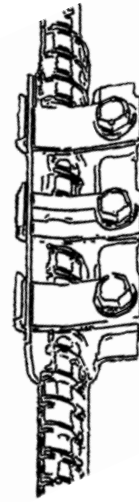
Figure 14 — Bolted strap coupling sleeve
